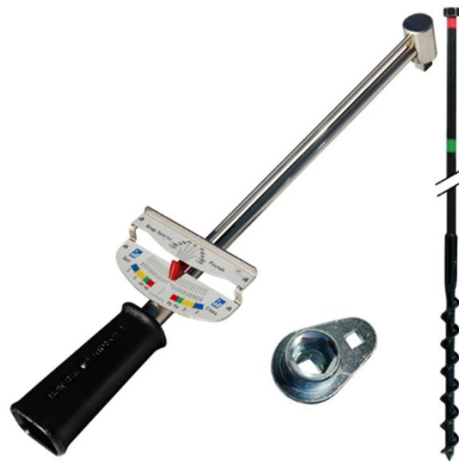
Figure 7. Soil test probe equipment.
